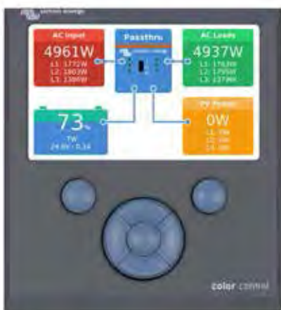
Color Control panel, showing a PV application
