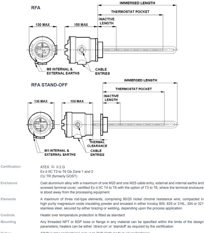
Rating 12kW (water applications) and up to 3kW (light-medium oil applications)
