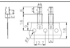
取付穴参考図 Size of Mounting Hole
